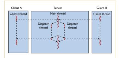
Figure 1. Synchronous call dispatch. Because the server uses a dedicated thread for each concurrent invocation, the clients tie up two additional threads for the entire duration of their blocking calls.
