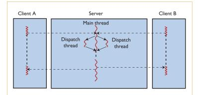
Figure 2. Asynchronous call dispatch. The server can implement any number of concurrent blocking calls using a single thread.
